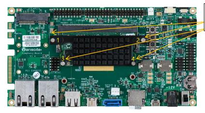
Heat sink alignment holes & screws
