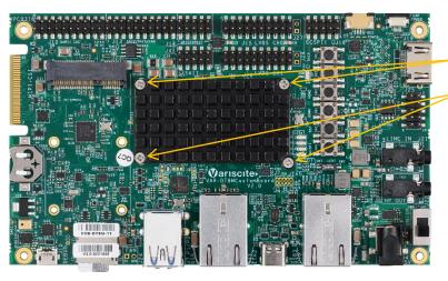
Heat Sink alignment holes & screws
