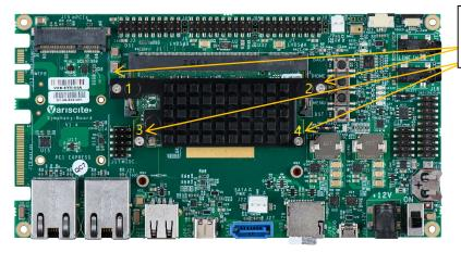
Heat sink alignment holes & screws
